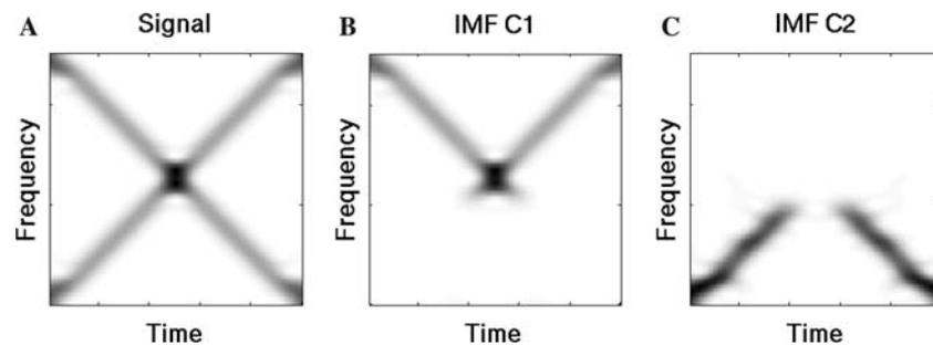
**Fig. 8** An example of EMD of a two-component signal. **a** The spectrogram of the composite signal that consists of two chirp components with opposite chirp rates and their time–frequency representations cross each other. **b, c** The spectrograms of the first two IMFs derived from the EMD, indicating the IMFs do not retain the original signal components. This example stresses that care must be taken in the physical interpretation of the decomposed IMF components
