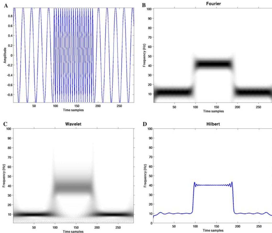
**Fig. 2** **a** A sine wave with abrupt changes of frequency around its midpoints. **b–d** Comparison between the short-time Fourier transform **b** the Morlet wavelet transform **c** and the Hilbert transform **d** The Hilbert spectrum reveals much sharper frequency and time localization compared to both the short-time Fourier transform and the Morlet wavelet transform. Note that some ripples in the Hilbert spectrum are due to the discontinuity in the data
