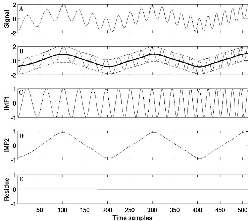
**Fig. 1** A simple example of the empirical mode decomposition (EMD) of a two-component signal. **a** The analyzed signal consisting a linear chirp and a nonlinear triangular waveform. **b** Upper and lower envelopes (*dashed lines*) of the original signal and its point-by-point mean of the envelopes (*thick line*). **c–e** Three IMFs from the signal. The EMD ends up with essentially two IMFs, each corresponding to the linear chirp and the triangular waveform
